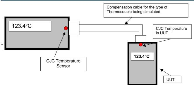
This method still requires characterised compensation cable for each type of thermocouple to be simulated. Additional uncertainties are introduced from the errors in using compensation cable between the UUT and the CJC in the calibrator. Also as the calibrator will have self-heating the error is greater due to the thermal gradient across the cable and plugs producing thermal emf.
