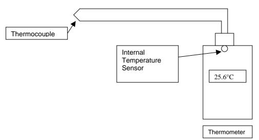
Inside the thermometer the CJC sensor is located as close as possible to where the metal of the thermocouple changes to copper, Note that thermocouples are supplied with special plugs (colour coded) made of the same metals of the thermocouple itself. If it is necessary to extend a thermocouple then it can only be extended with the same metal. The whole effect of a thermocouple is due to connecting different metals together, so great care must be taken to avoid large errors.
