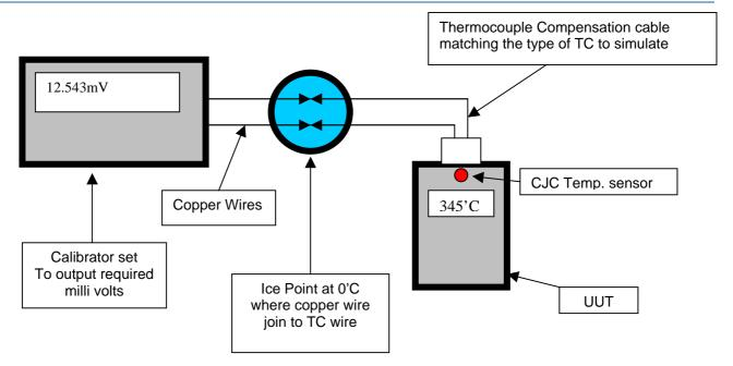
This method is accurate, but requires an ice point reference and also characterised Thermocouple compensation wire is needed for each type of TC to simulate.
